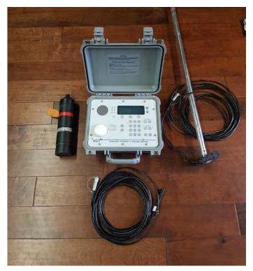
**Figure 5-23.** Acoustic telemetry tracking equipment used in the 2016 Dungeness crab study: Vemco VR2W stationary receiver/logger (left), Vemco VR100 acoustic receiver (center), pole mounted Vemco VH110 directional hydrophone (right), and Vemco VH165 omni-directional hydrophone (bottom).
